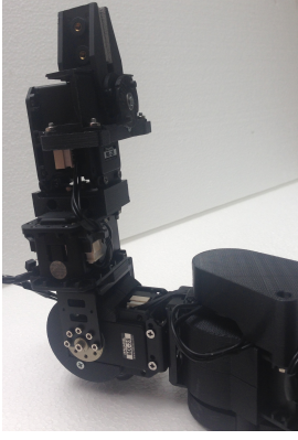
Fig. 1. Robai Cyton Gamma robot arm, two joints
